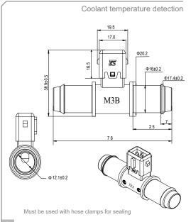
Feature | Designed for mating with elastomeric hose
